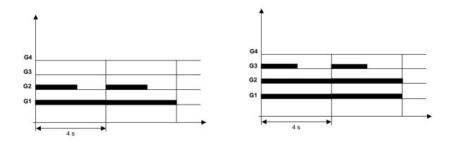
In case of simultaneous request of heating and tank, the controls G1-G4 related to the main heat exchanger will be directed in the following way:
